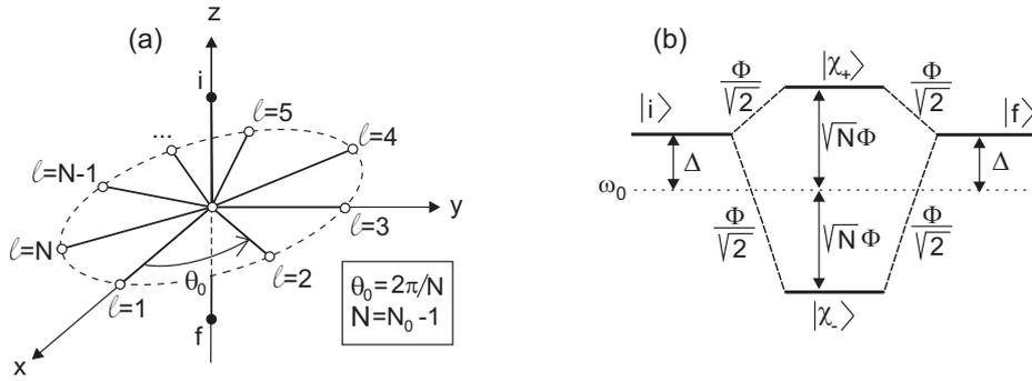
**Fig. 2** (a) Representation of two defect sites  $i$  and  $f$  connected to the central core of a star graph  $S_N$  with  $N = N_0 - 1$ . (b) Representation of the restricted Hamiltonian  $\mathcal{H}$  that governs the exciton dynamics when the input site is initially excited (see the text).
